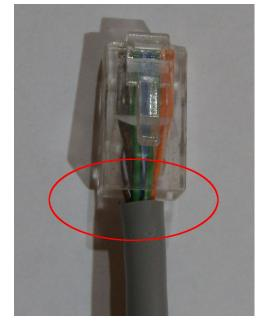
This is an example of wires that are okay. The sheath fits well into the ice cube.
